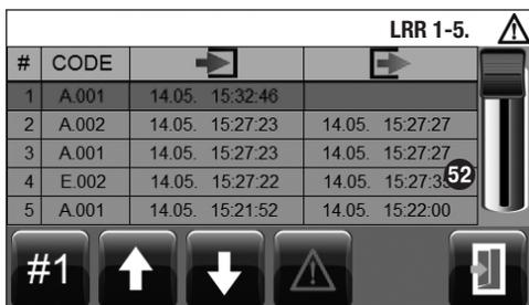
The active alarm or malfunction is highlighted in red. Press button
