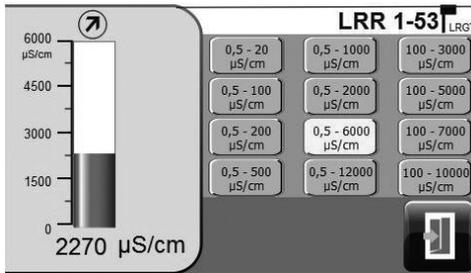
The factory-set measuring range is shown. If required press the button for your required measuring range.
