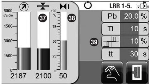
For each parameter setting press the green button. Use the on-screen numberpad to enter the desired value.
