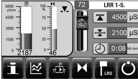
Use the hand slider to change the position of the continuous blowdown valve. The green button indicates the valve opening in %. Or press the green button and enter the desired valve opening in % in the numberpad.
